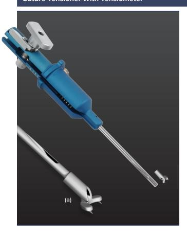
The suture tensioner with tensiometer allows simple, reproducible graft tensioning intraoperatively for both transtibial and all-inside ACL/PCL reconstruction. The footpiece may be used to secure the tensioner around the tibial tunnel, allowing placement of an interference screw during tensioning. Remove the foot to simultaneously tension and tie graft sutures over a button or suture post.
